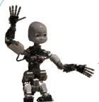
Developmental robotics systems start with little or no information about the surrounding scene. The cognitive architecture of the iCub humanoid robot (53 degrees of freedom) aims at understanding environment with increasing degree of precision.
